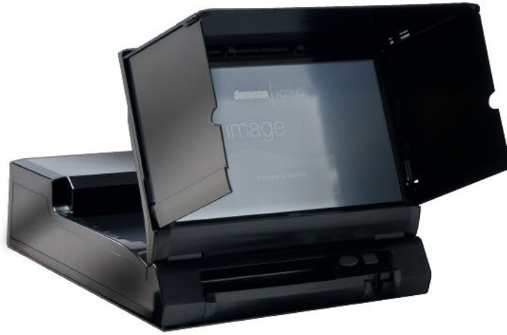
Figure 2.4: The ImageCast® Evolution Ballot Counter in Operating Position.
